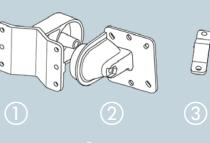
Screw the connector flange (2) to the back of the housing with the four screws and their washers.
