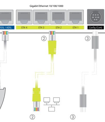
Ethernet interface Use the cable with the green-colored connectors to connect one of the interfaces ETH 1 to ETH 4 to your PC, IP telephone or a LAN switch.
