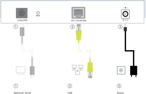
**Optional: Serial** configuration cable You can connect the device to a PC with a configuration cable (available separately).
