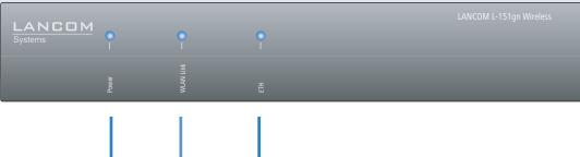
Device switched off Device operational (permanently) Configuration password not set. Without a Blinking green configuration password, the configuration data in the device is unprotected.
