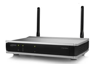
The LANCOM L-151gn Wireless is a professional 11n WLAN premium entry access point. It serves 11n clients with professional and reliable WLAN in the 2.4 GHz frequency band and is therefore the ideal entry device for the business field in LANCOM premium quality.
