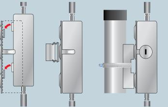
Align the four openings on the rear of the device housing with the clips on the base plate and snap-fit the
